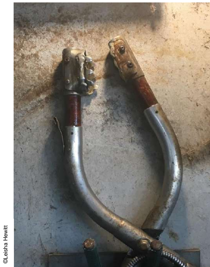
Figure 12. Worn and therefore unsuitable stunning electrodes
