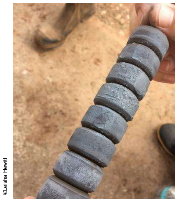
Figure 11. Build-up of residue around the recuperator sleeves
