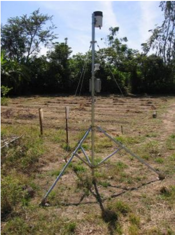
Figure 17 Automated met station in Adi Ha Nursery with manual raingauges in background
